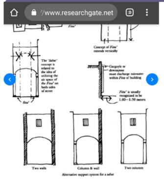
The Fina and Sabat . The diagram shows how the Fina is utilized. It is an invisible space about 1.00– 1.50 m wide alongside all exterior walls of buildings – primarily alongside streets and access paths – and extends vertically alongside the wall of the building. The principle for the formation of the Sabat is shown as well as various methods for its support. Drawing by the author from Hakim, (1986).<sup>14</sup>
